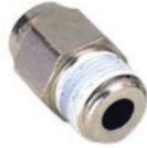
92707 Slip-Lok × MNPT adapter 3/8" Slip-Lok × 3/8" MNPT · two per ring
