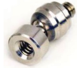
Swivel adaptor Nozzle swivel adaptor 10/24 thread · 30° swivel · finger- tight
