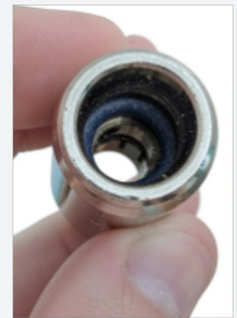
O-ring placement inside the Slip-Lok, which the collar seats against.
