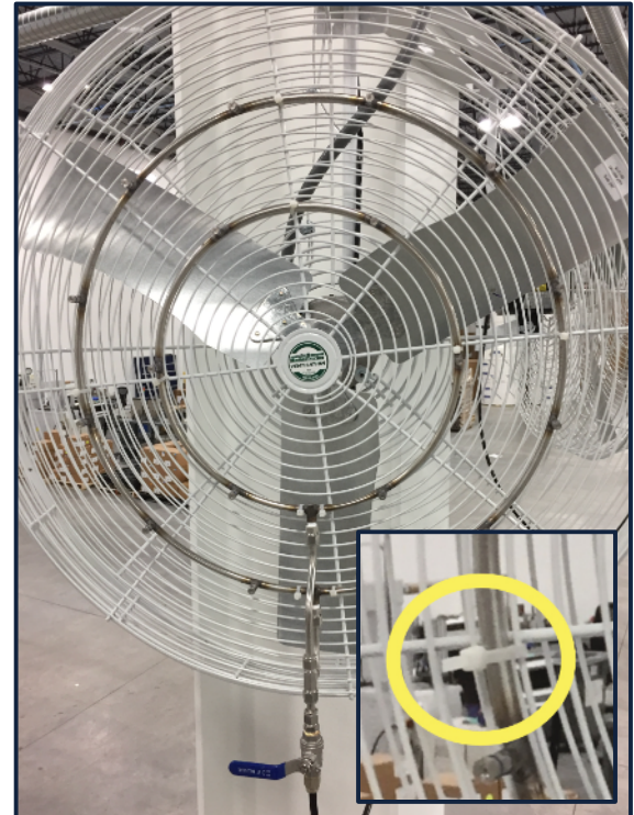
Fig. 9.1 MIST-RING INSTALLED Secured with 5 zip ties – centered on the fan face guard
