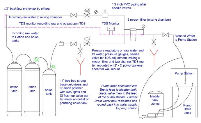
The Service Technician installs the anion and cation tanks, the wall mount blending panel, the bladder tank functioning as an expansion chamber, and sets TDS to your desired setting (generally 50 ppm). To set the system in operation, the technician sets the raw water regulator to 40 psi and sets the DI pressure to 30 psi. then adjusts TDS as displayed by the TDS monitor to pump station with the raw water needle valve.
