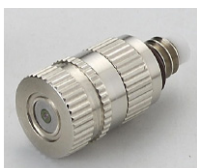
SS High Pressure Nozzle Part # IHC-10.58 "Colorless" Band 0.3 mm / .012" orifice 0.021 gpm / 10.58 lbs/hr
