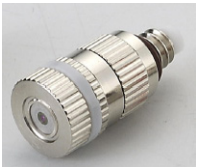
SS High Pressure Nozzle Part # IHC-3.97 White Band 0.1 mm / .004" orifice 0.0079 gpm / 3.97 lbs/hr
