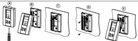
CAUTION: Risk of malfunction. Remove power prior to separate humidistat cover from its base.
