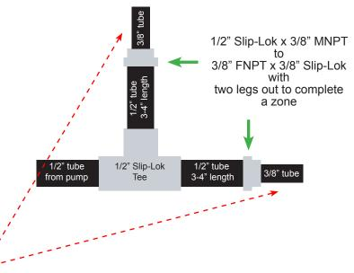
At a transition junction, it may be considered to install a 3/8" ball valve to have control points to shut off water to each leg if ever necessary.
